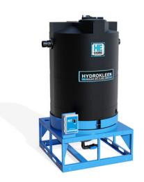
separation and solids settling. Clarified liquid is skimmed from the surface at the discharge point. Solids accumulation at tank cone bottom are either periodically purged for downstream accumulation or optionally pumped to a Hydrokleen CMAFU-2 for filtration.
